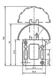
Arch profiles made of UHMW, PE Max load (25C) 130N
